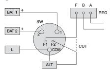
Two Engines and Two Batteries, with Battery Isolator
